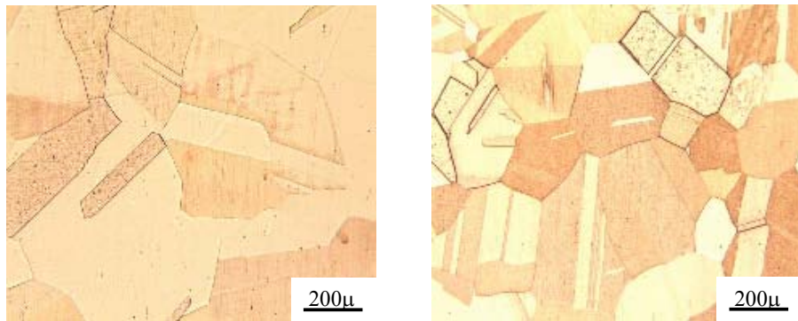
Figure 5. Optical micrographs of the brass sheets for the 0.25/800°C route: (a) as-received and (b) annealed conditions.
