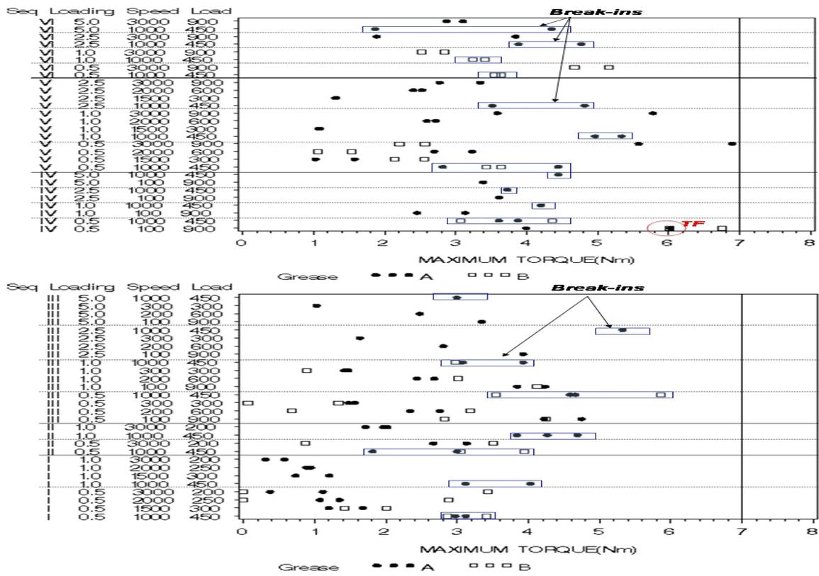
Figure 4. Maximum torque responses for A & B.
