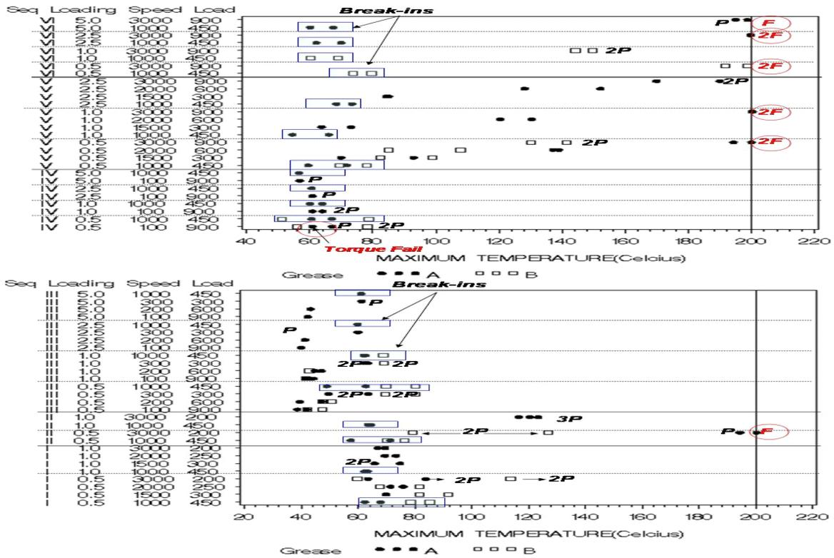
Figure 3. Maximum temperature responses for A and B.
