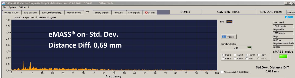
Figure 2. eMASS® effects on the frequency distribution and the standard deviation of strip vibrations at GalvTech, Pittsburgh, USA, 2012 (top image: eMASS® off / bottom image: eMASS® on).
