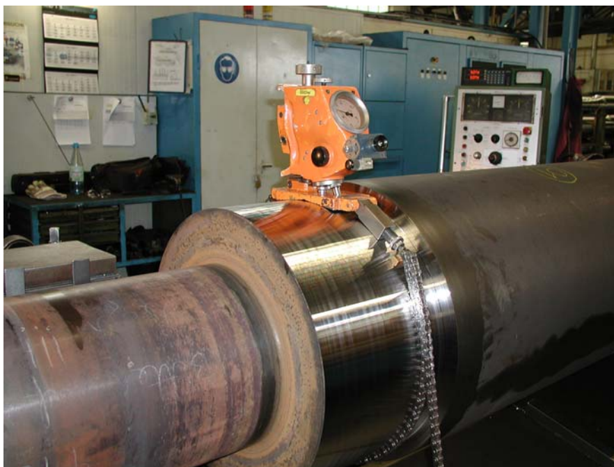
Figure 3. Experimental setup to determine the real hardening depth of a roll.
