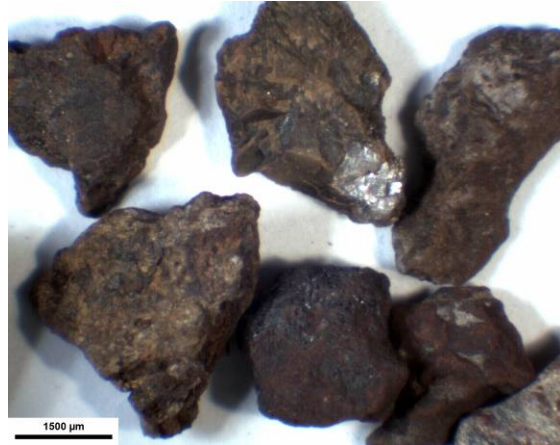
Figure 4. Ore 2, fraction -6.35+3.36 mm. Once more iron oxi-hydroxides and gangue mineral associations.
