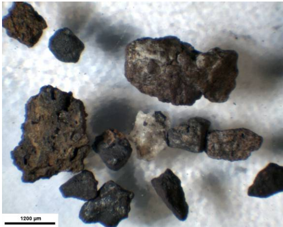
Figure 5. Ore 2, fraction -3.36+1.19 mm. The presence of quartz practically in free particles is observed in this fraction.
