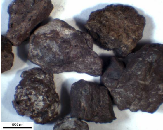
Figure 3. Ore 2, fraction -6.35+3.36 mm. Details of iron oxi-hydroxides and gangue mineral associations.
