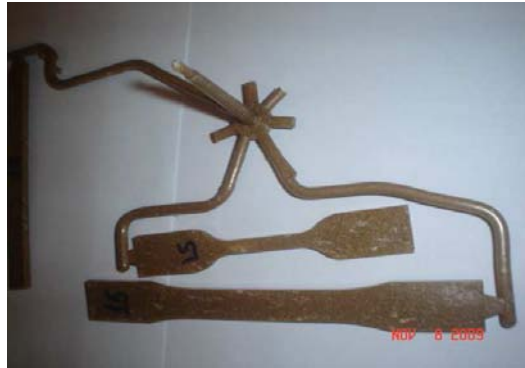
Figure 1. Injection molded test specimens
