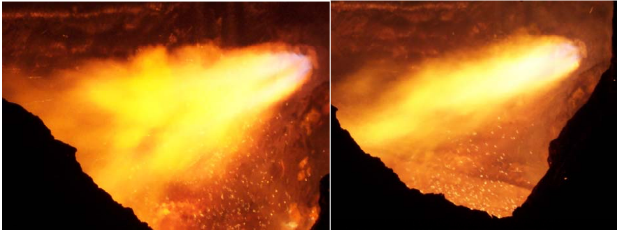
Fig. 7- DanHELIOS ® flame characteristics - turning from large to concentrated flame.
