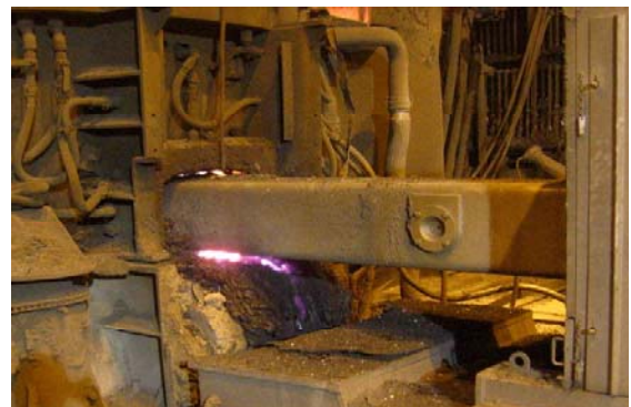
Fig. 12 - Sill level cleaning robot
