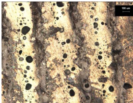
Figure 4. Micrography of the alloy Al-1.5wt%Fe treated by laser surface remelting processes.
