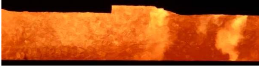
Figure 8: Highly diluted flames created by the REBOX HLL installation at the walking beam furnace in SSAB-Borlänge in Sweden. The fuel used is heavy oil.
