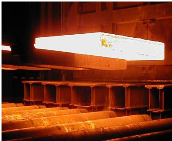
Figure 14: Outokumpu in Sweden increased its heating capacity in the existing walking beam furnace by >35% when implementing flameless oxyfuel.
