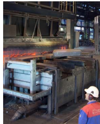
Figure 14: Outokumpu in Sweden increased its heating capacity in the existing walking beam furnace by >35% when implementing flameless oxyfuel.
