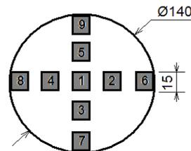
**Figure 1.** Specimens position for the characterization of ductile cast iron.
