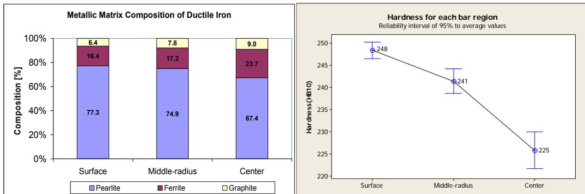
**Figure 3.** (a) Proportion of constituents of metallic matrix and (b) Average hardness of ductile cast iron as a function of analyzed region.
