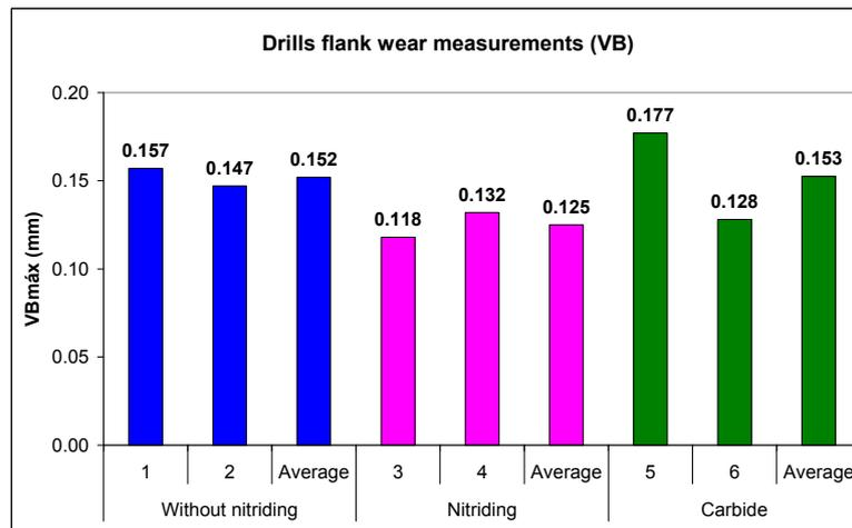
Figure 4. VB maximum values observed in the drills.
