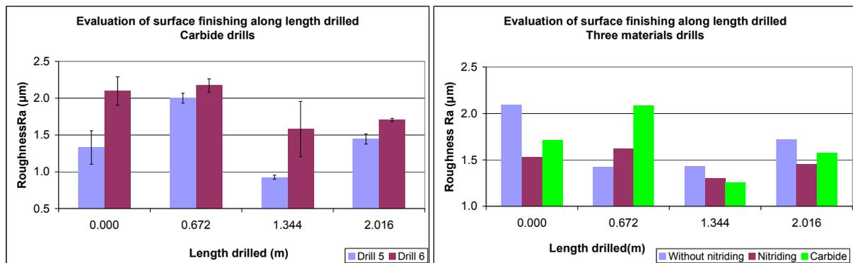
**Figure 7.** Variation of roughness Ra drilled along the machining length: a) Drills Carbide b) Comparison between the three types of drill.
