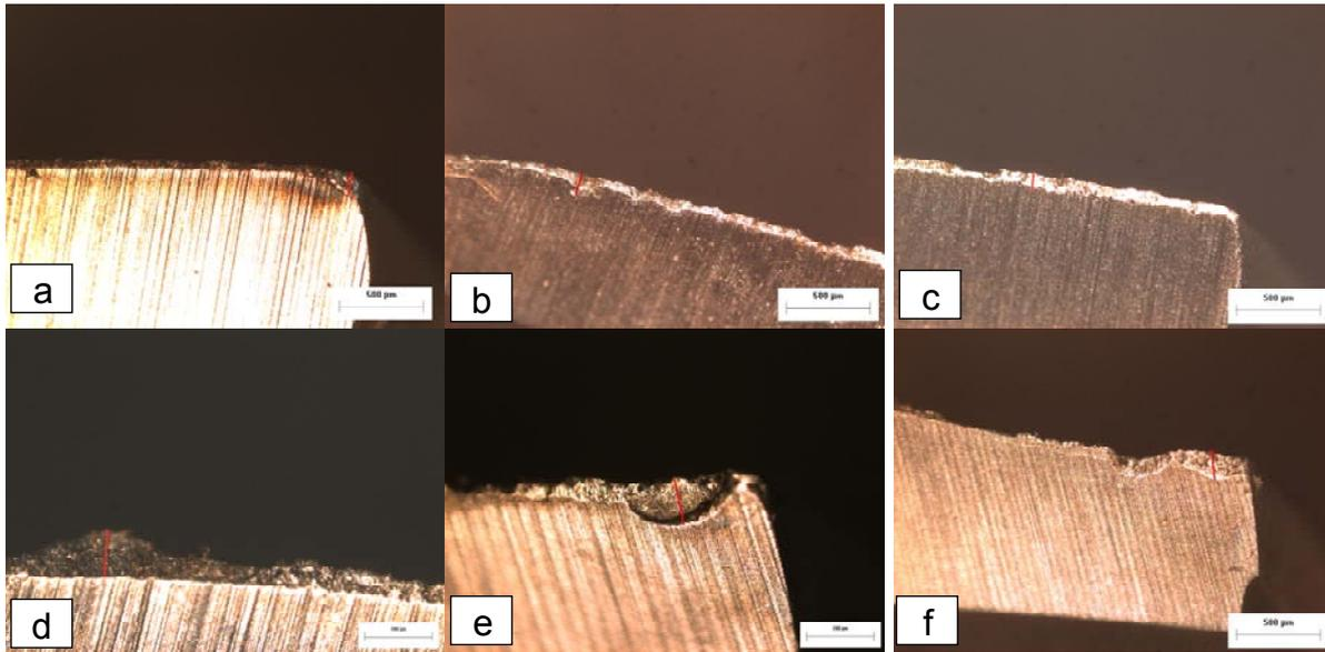
**Figure 5.** Flank wear observed in drills [a,b] without nitriding, [c,d] nitriding and [e,f] carbide.
