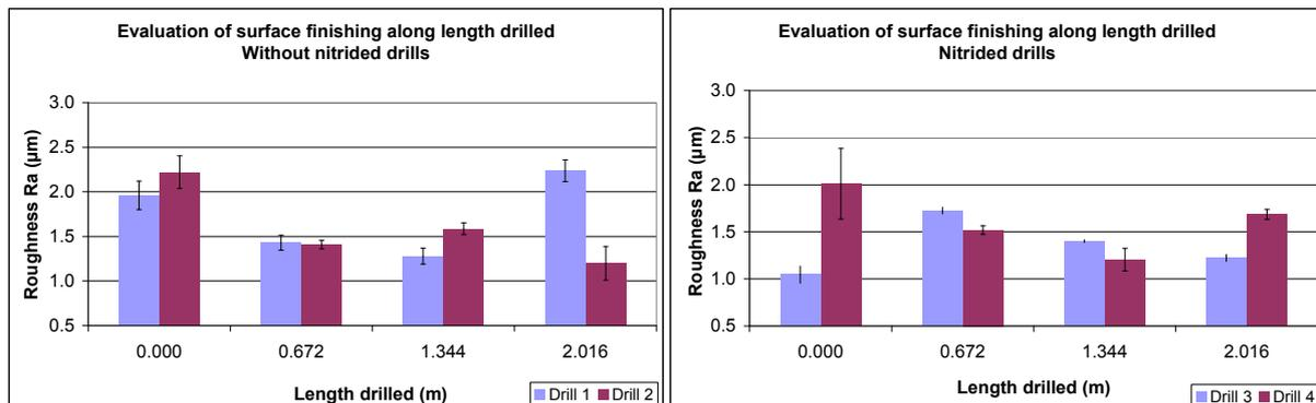
**Figure 6.** Average surface roughness variation along the length drilled using drill: a) without nitriding and b) nitrided drills.
