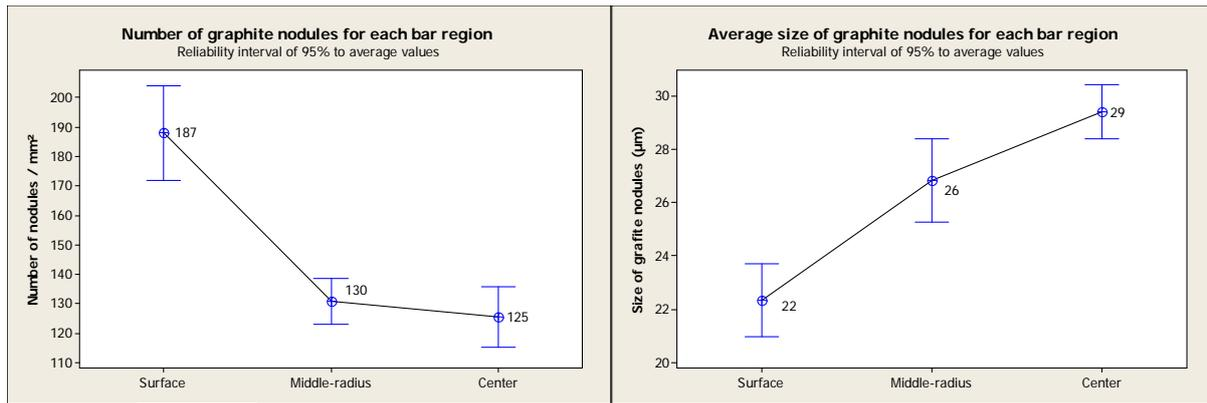
**Figure 2.** (a) Number of graphite nodules and (b) Mean size of graphite nodules.
