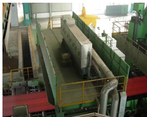
Figure 9: Rometer F100-2P gauge at mill exit.
