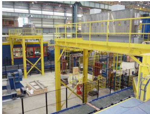
Figure 10: Rometer FQC-2 gauges at cold leveller exit (2 lines).
