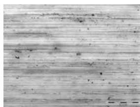
(a) Cilindro #3 Superior Rug Ra: 20,3 μinch
