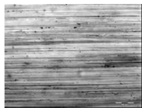
(c) Cilindro #4 Superior Rug. Ra: 10,7 μinch
