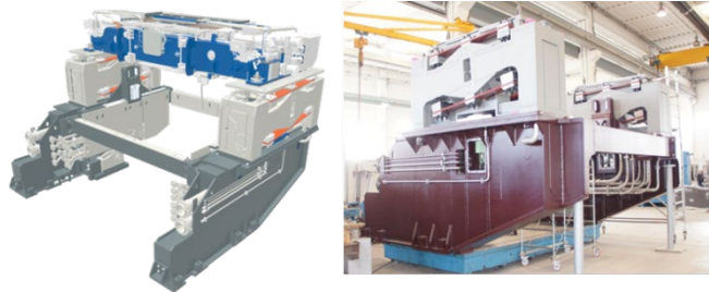
Figure 9. Resonance oscillation system, hydraulically actuated
