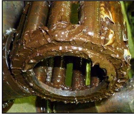
**Figure 8.** Steel mill guide bearing lubricated with a calcium sulfonate grease.
