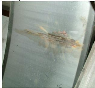
**Figure 1.** Corrosion shown on a work roll bearing
