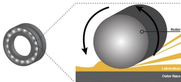
**Figure 5.** Schematic diagram of EHL.
