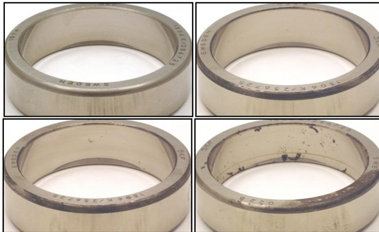
**Figure 3.**Example of an EMCOR rust test for high-performance mineral gear oils (Oil A on the left, Oil B on the right).
