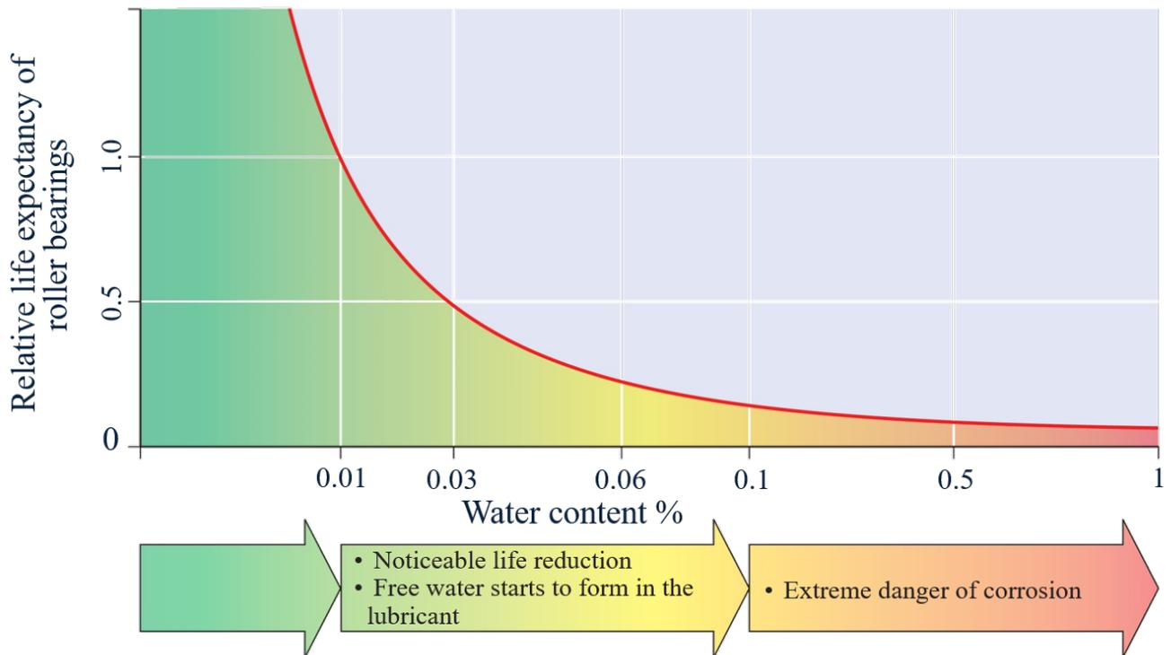
Figure 2. Relative change in roller bearing life expectancy as water content increases.
