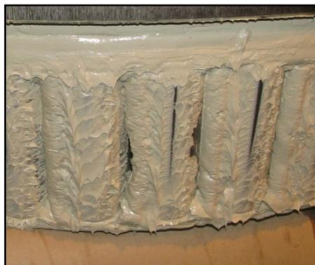
**Figure 7.** Reversing mill backup roll bearing lubricated with a calcium sulfonate grease.
