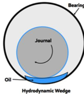
**Figure 4.** Schematic diagram of hydrodynamic lubrication.
