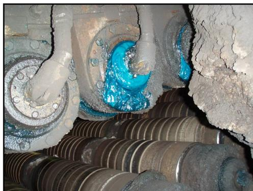
**Figure 6.** Example of continuous caster roll bearing using a lithium complex grease.
