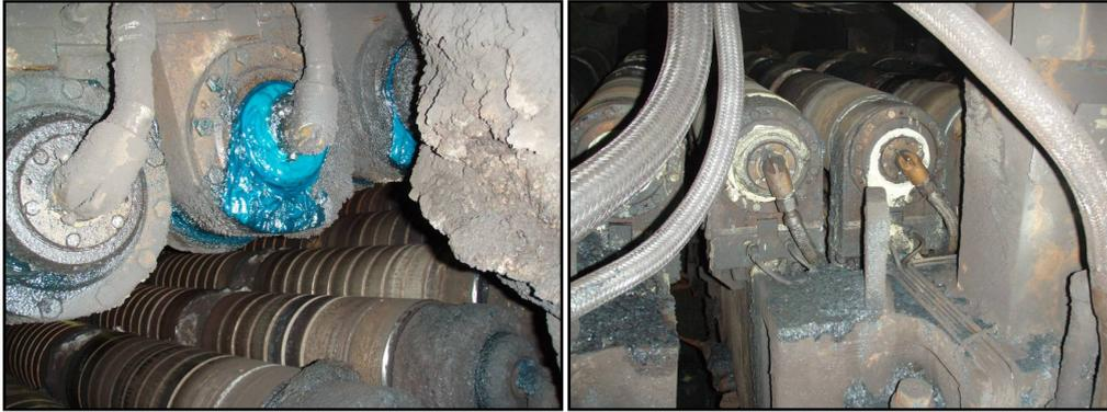
**Figure 9.** A continuous caster bearing lubricated with a lithium complex grease (left) compared to one lubricated with a calcium sulfonate grease (right).
