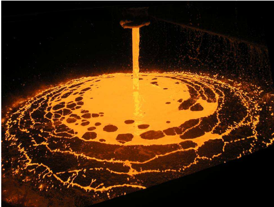
Figure 3 - Granshot granulation on sprayhead - typical metal umbrella formation.
