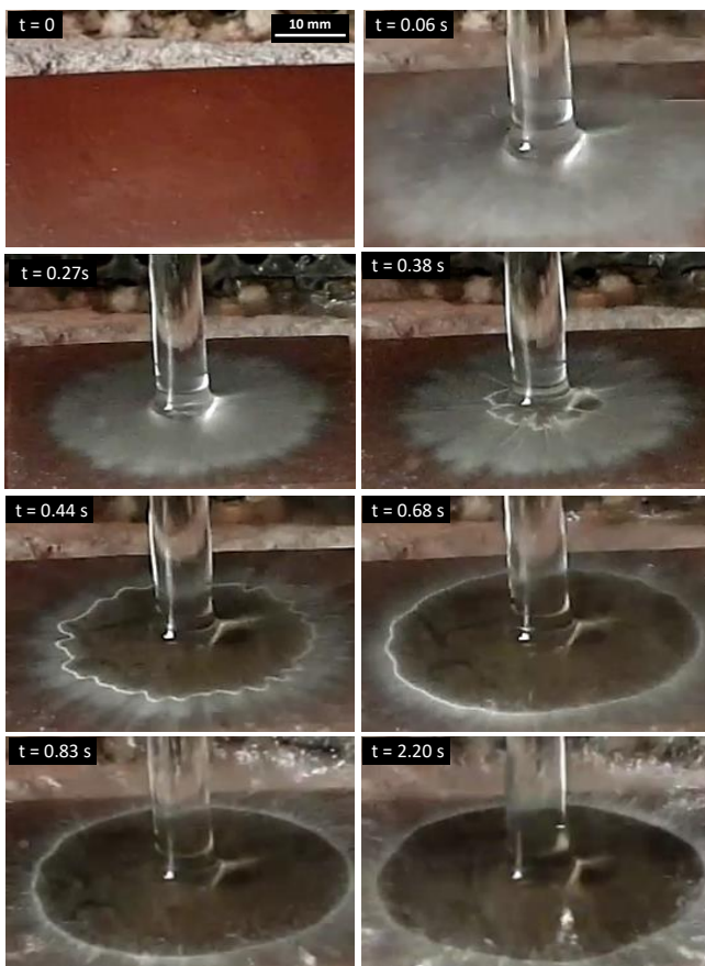
Figure 3. Sequence of events of the wetted region growth for T_i = 896^\circ\text{C} and T_j = 20^\circ\text{C} .
