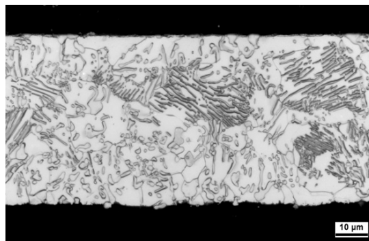
Figure 1. Initial microstructure of C100, soft annealed, Nital etch (3%) for 25 s.
