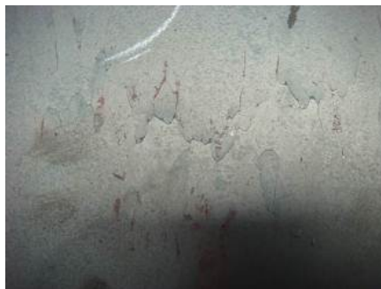
Figure 7. Example of surface defects from hot shortness caused by copper contamination from casting mold. Note this is not the same type of defect as seen in star cracks.
