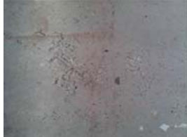
Example of thermal shock cracking on the top surface of heavy gauge rolled plate from cold scarfing of high CE slab
