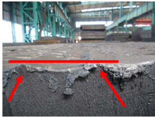
Example of good scarfing technique with proper scarfing depth to width ratio (feathered technique).
