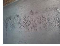
Example of thermal shock cracking on the top surface of heavy gauge rolled plate from cold scarfing of high CE slab
