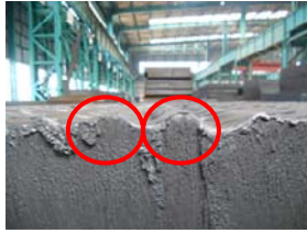
Example of poor scarfing technique, too steep
