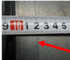
Example of straight away rolled scarfing defect from poor edge scarfing technique
