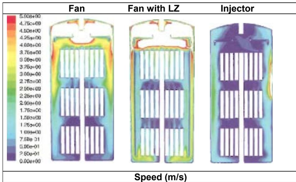
Figure 2. CFD vector field in a pit furnace (D 900 mm, H 2000 mm); the Simulation calculation for the process with fan in Operation shows a much more inhomogeneous flow field.
