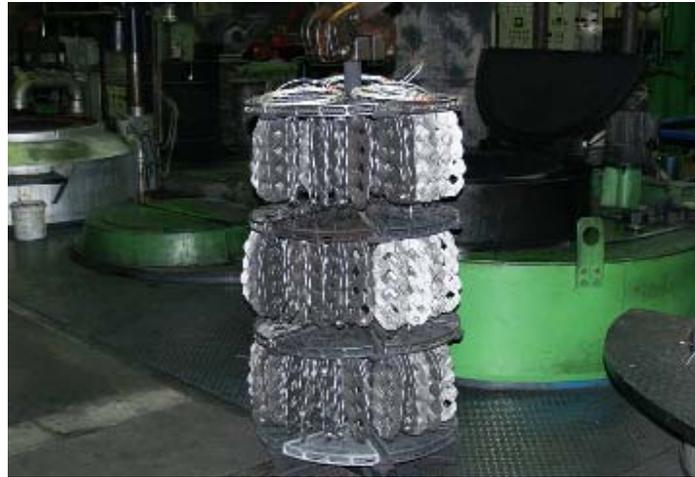
Figure 3. Pit furnace with reference charge.
