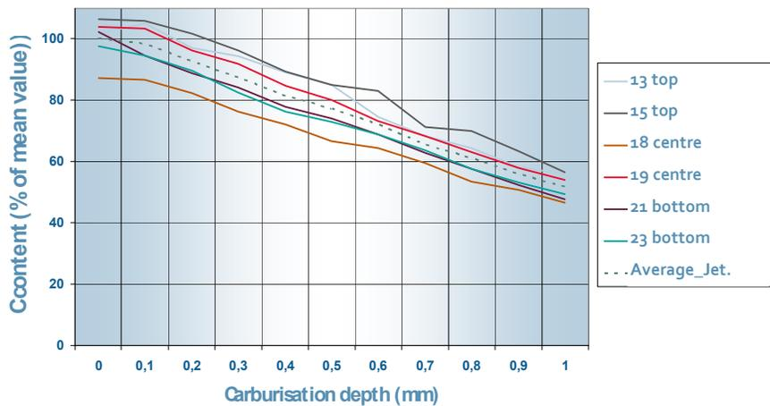
Figure 6. Carbon depth profile in 16MnCr5 test samples in process with fan, analysed by GDOS.
