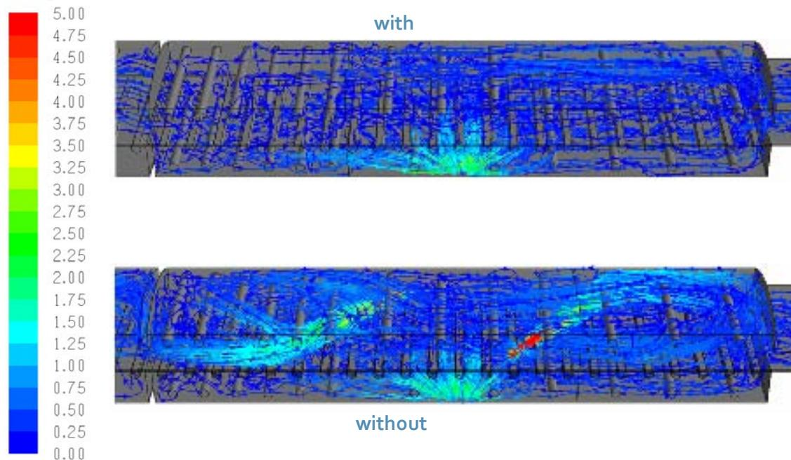
**Figure 10.** a) Gas velocity (m/s) in the zone of endogas injection into a roller hearth furnace. The main velocity is relatively low. A definite increase can be shown at the endogas inlet only. b) Gas velocity (m/s) in the zone of endogas injection into a roller hearth furnace with 2 CARBOJET<sup>®</sup>-lances. The total gas velocity is significantly higher whereas the red colour stands for particularly high values. The total gas consumption is equal for both simulations.
