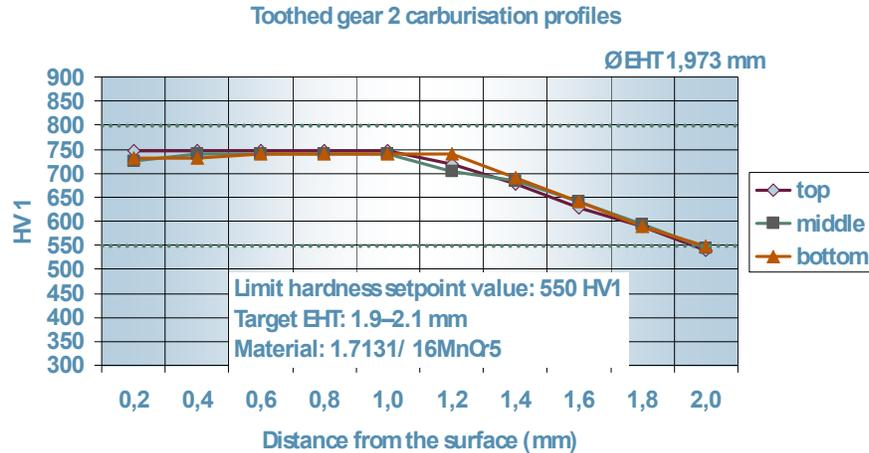
Figure 8. Practical results for carburizing depth 1.9-2.1 mm.
