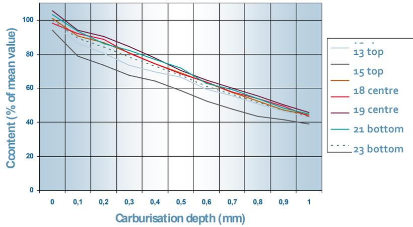
Figure 5. Carbon depth profile in 16MnCr5 test samples in process with CARBOJET®, analysed by GDOS.
