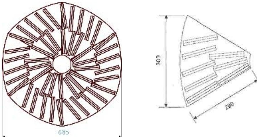
Figure 4. Allocation of ballast, 288 pieces of ballast, 0.635 kg each, total of 183 kg.
