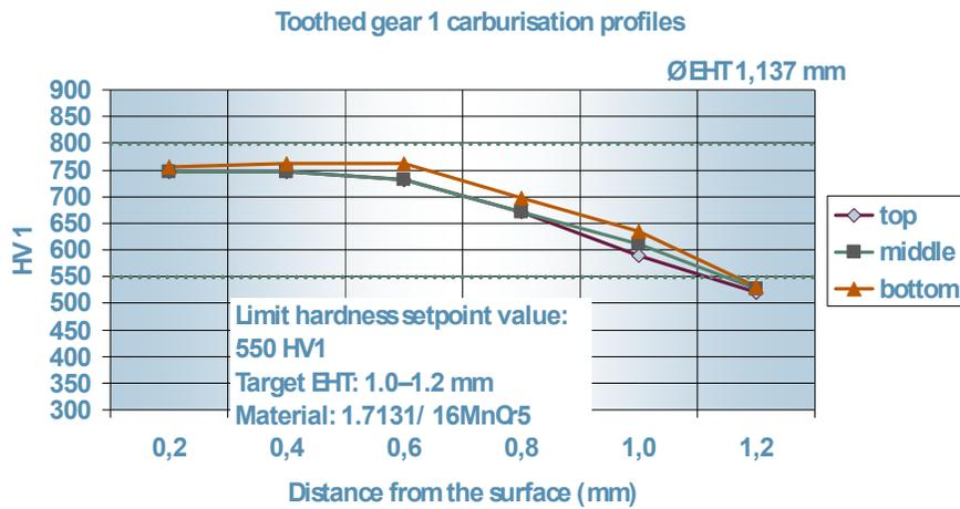
**Figure 7.** Practical results for carburizing depth 1.0-1.2 mm.
