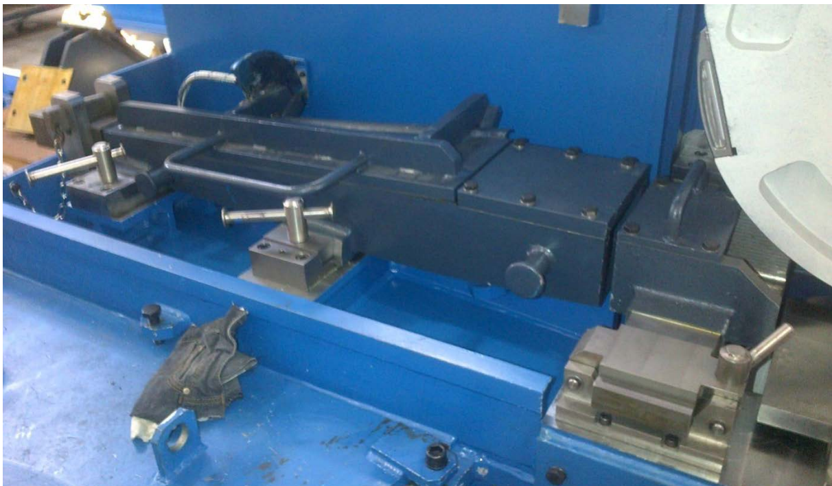
Figure 1. HSS II Generation: equipment mounted directly on shear foundation.
