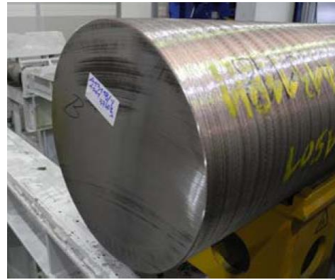
Figure 14: electrode with a 45° chamfer
