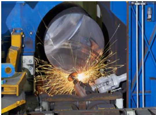
Figure 13: grinding robot in operation
