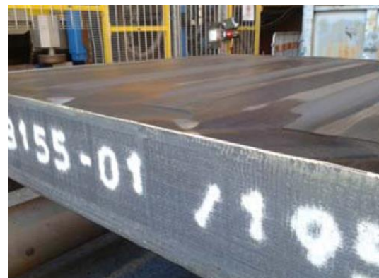
Figure 12: Longitudinal Deburring Grinding Results
