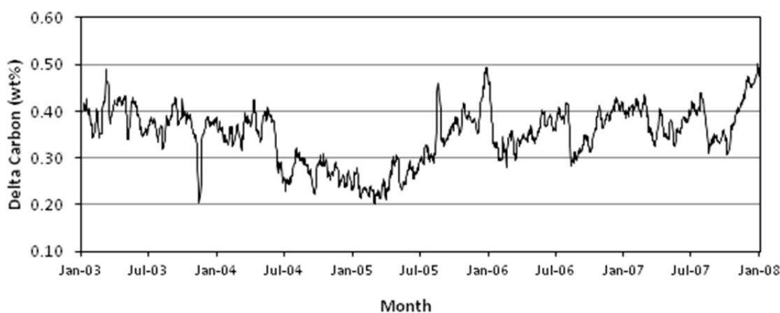
Figure 10. \Delta C trend for No.6 Blast Furnace 2003-2008.
