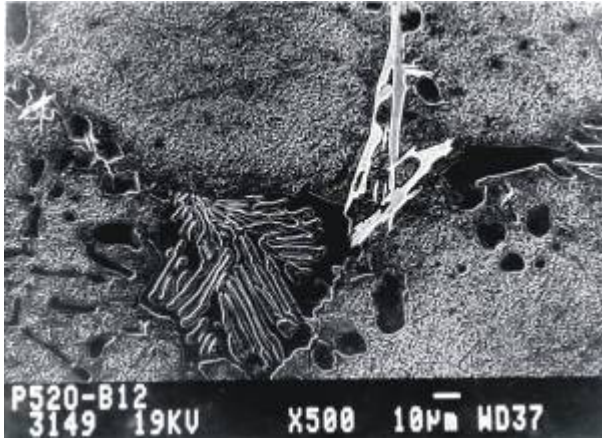
Figure 1a. Cluster of MC (black lobules), M_2C (platelike) and M_7C_3 (black fan-shape) in Kosmos grade (martensitic matrix)
