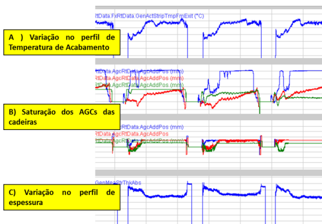
Figure 8. Effect of temperature variation on thickness temperature profile
