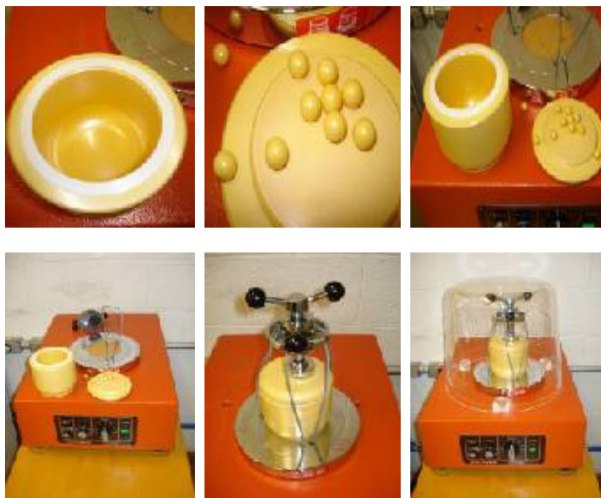
Figure 3. Picture of the ball milling step of the preparation process of the LSM by solid-state method.
