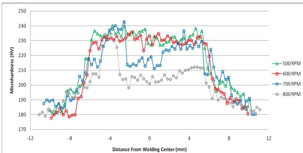
Figure 5. Comparison of hardness profile FS welded samples welded with different energy inputs.
