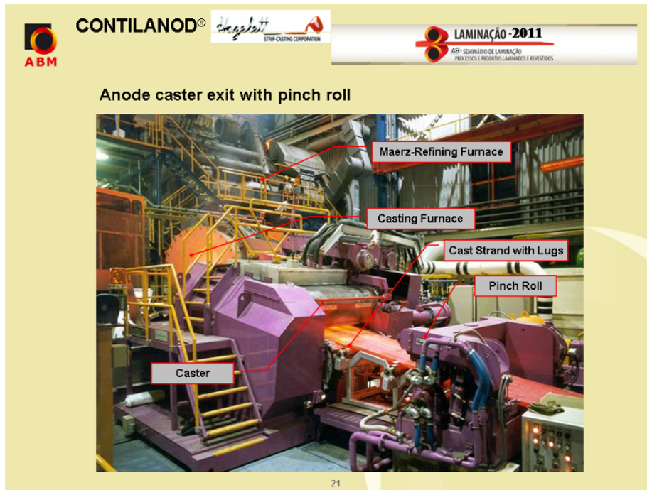
Figure 8. Hazelett anode caster at MKM line.
