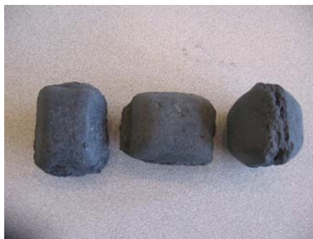
Figure 17: Example of (MgO-Carbon) foaming slag enhance “Pro-Slag® [9] slag additive compound” briquettes - dimension “~ 40*20*20 mm”
