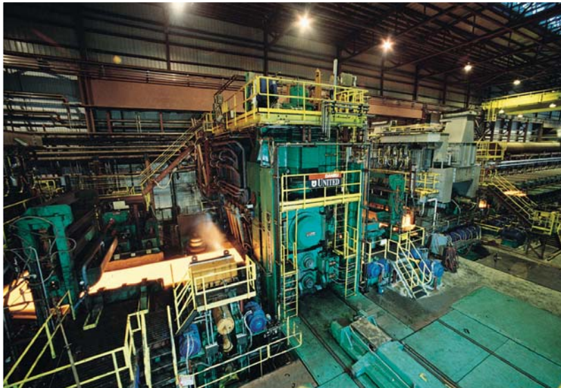
Figure 3 - 4-Hi Steckel reversing stand
