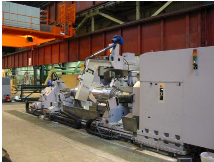
Figure 1. Cold Mill Roll Grinder with integrated shape measurement system.
