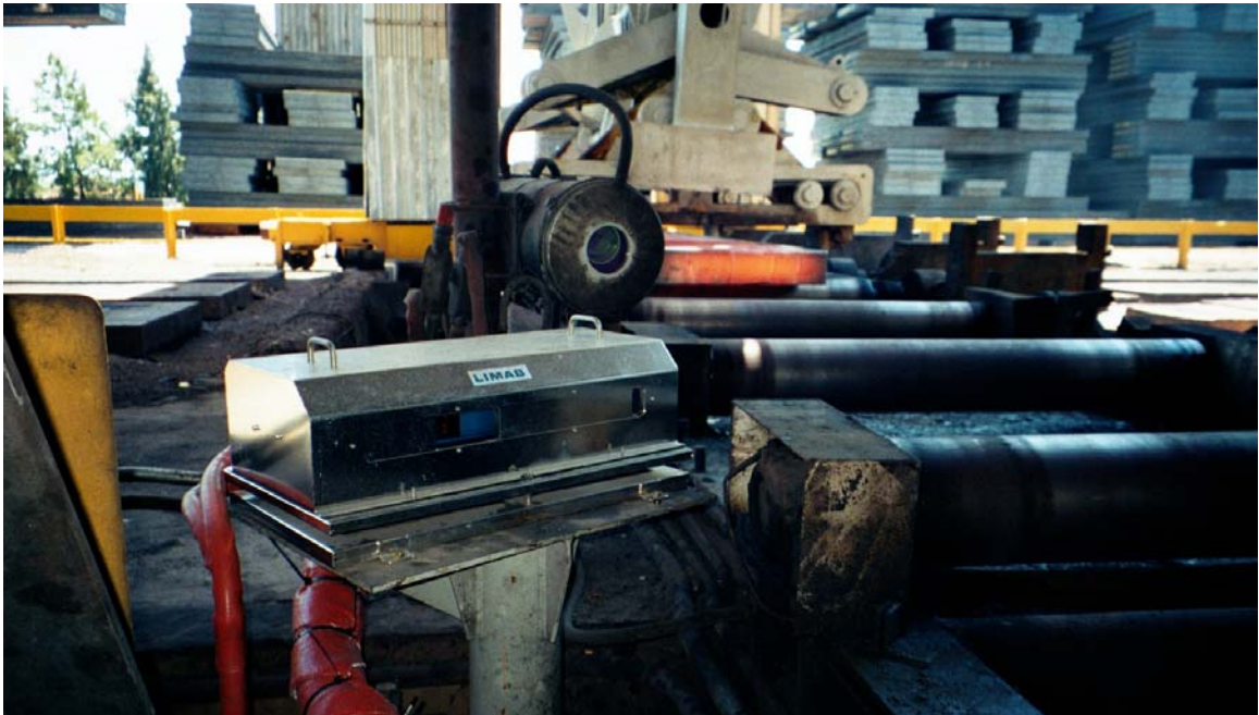
Figure 4. Length measurement sensor in stainless steel cooling box (courtesy of Siderar, Argentina)
