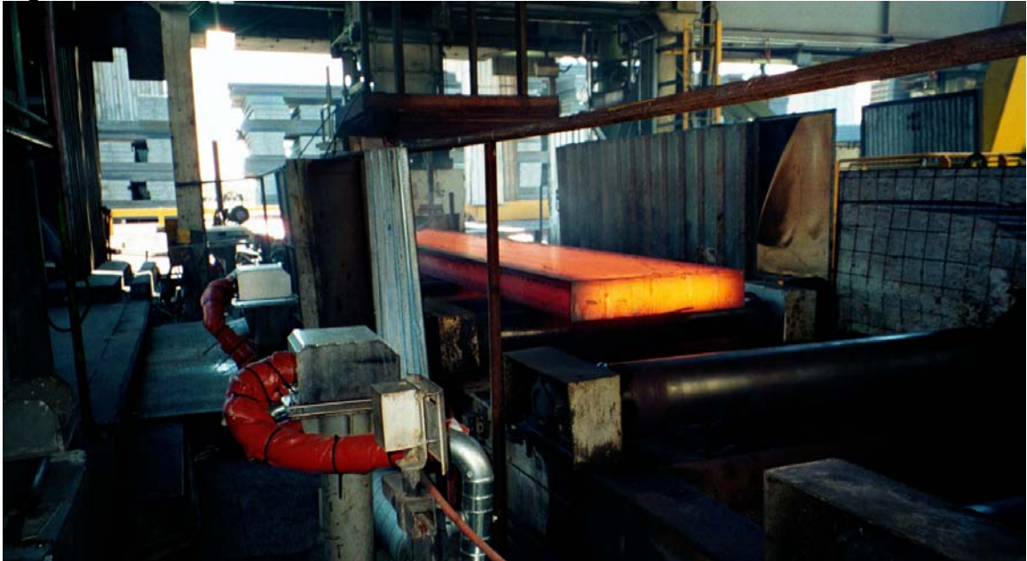
Figure 3. Photocell transmitters and length measurement sensor in the far back ground (courtesy of Siderar, Argentina)
