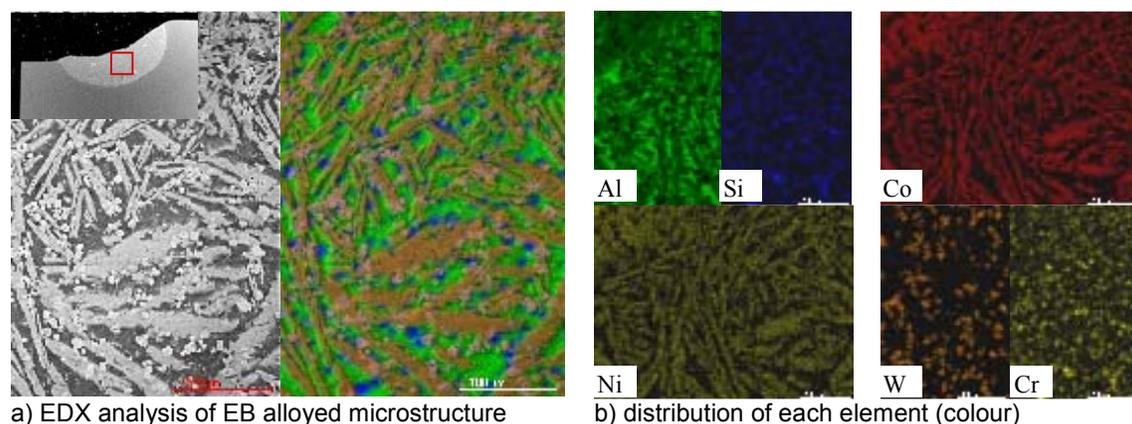
**Figure 3.** EB alloyed layer with Co additive (base material: AISi21Ni7Cu3).
