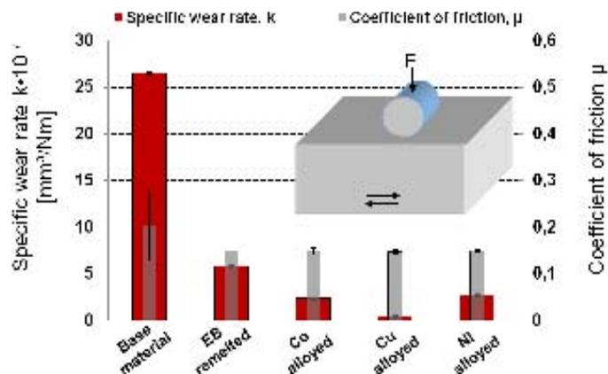
**Figure 5.** Results of fretting wear tests of AISi35 under oil-lubricated conditions at  $T = 80 \text{ }^\circ\text{C}$ .
