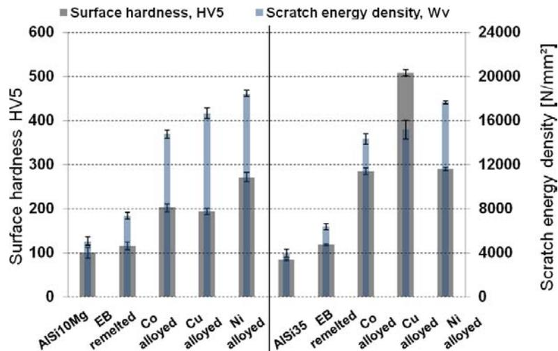
**Figure 4.** Maximum surface hardness and scratch energy density of AISi10Mg and AISi35 untreated and remelted state and in dependence of alloying additives.
