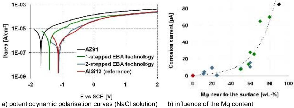
**Figure 8.** Corrosion behavior – influence of EB technology / content of Mg near to the surface.
