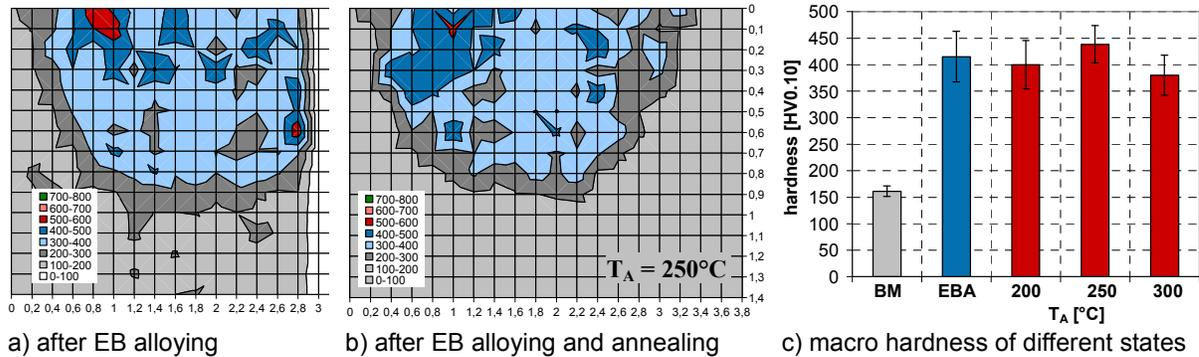
Figure 6. Hardness distribution [HV0.10] of EB alloyed layer (EBA) with Co additive (AlSi21Ni7Cu3).
