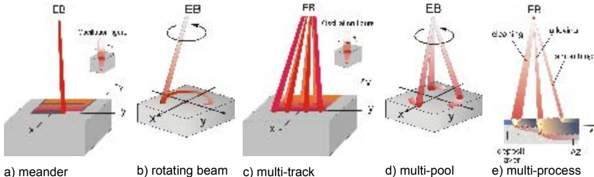
Figure 2. EB surface treatment with a, b) one- and c, d) multi-spot technique or e) multi-process technique.
