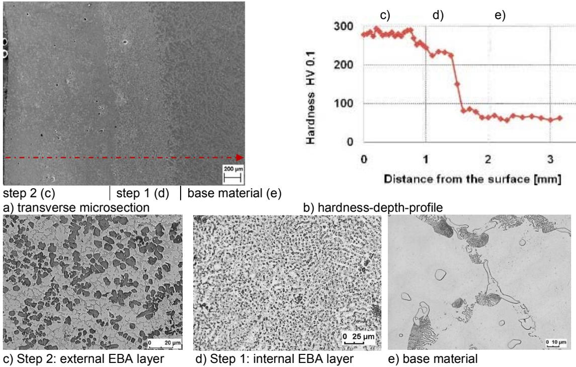
**Figure 7.** Local microstructure and microhardness profile after a two-step EBA double process.
