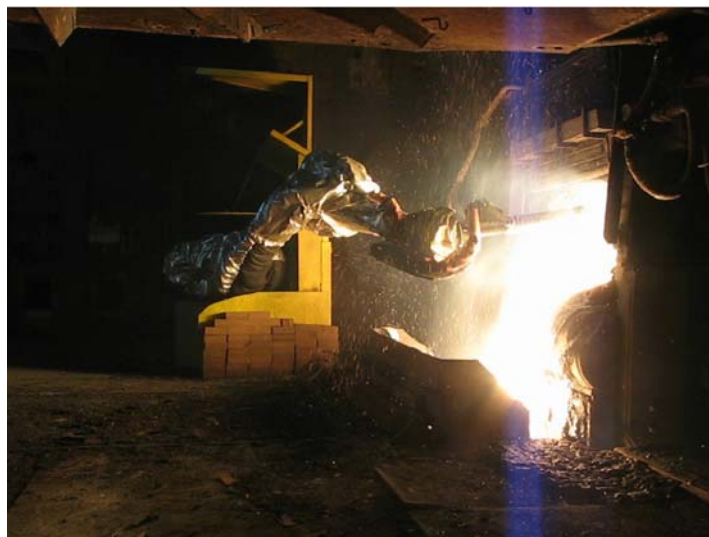
Figure 4: LiquiRob ® during oxygen measurement operation in EAF.
