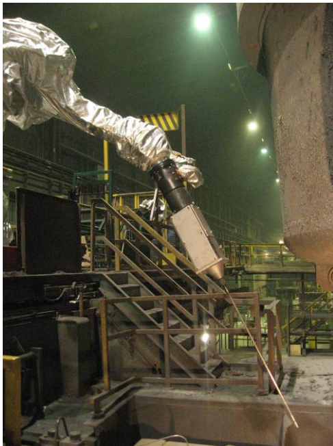
Figure 6: CCM5 Layout and pictures of measurement and oxygen lancing position.
