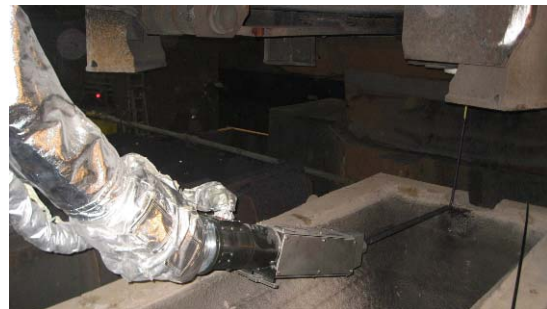
Figure 6: CCM5 Layout and pictures of measurement and oxygen lancing position.
