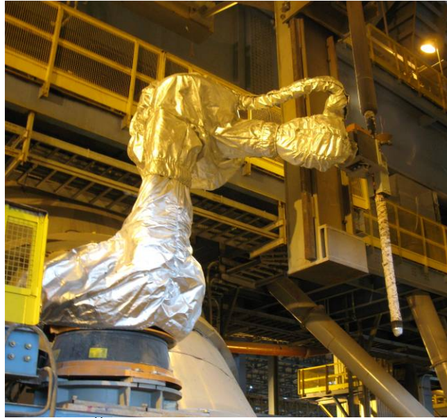
Figure 5: LiquiRob ® disconnecting a probe cartridge from the substance
