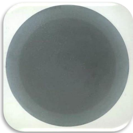
Figure 8: Macrography after quenching.
