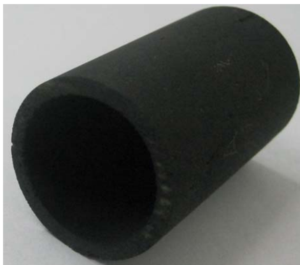
Figure 1. Prototype of AC composite membrane used in the research.
