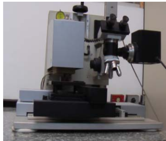
Figure 2 – (a) schematic representation of head system measurement of a Fischerscope H100V machine: 1) electro-magnetically load system; 2) force; 3) displacement sensor; 4) motor; 5) indenter; 6) reference ring; and 7) specimen; (8) (b) Fischerscope H100V machine.
