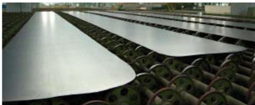
Figure 8: Thanks to PFC from Siemens, these plates with a thickness of 5.3 mm show excellent flatness on the cooling bed.
