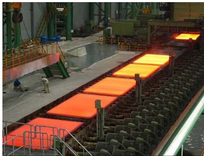
Figure 4: Picture of a batch produced with automated batch rolling.
