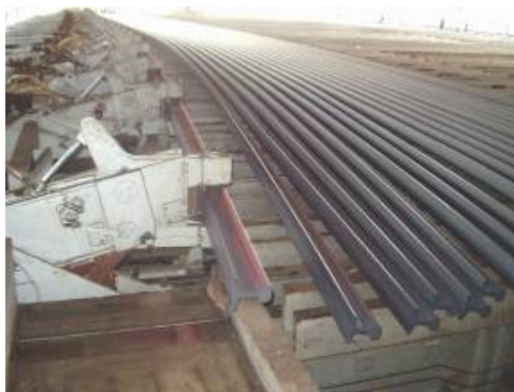
Figure 12. EVO pre-cambering system.
