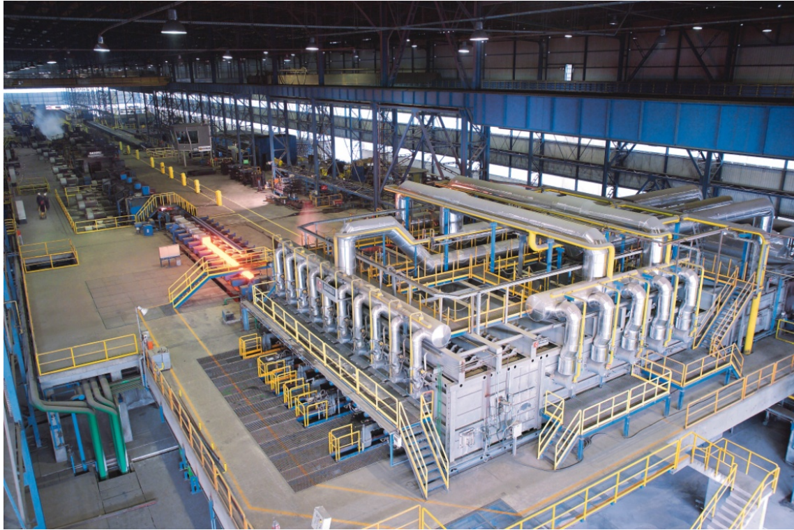
Figure 12. Reheating Furnace with pulse firing technology
