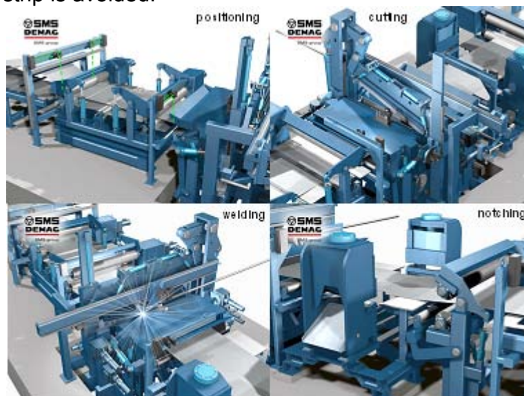
Fig. 12: Welding cycle of the new welding machine
