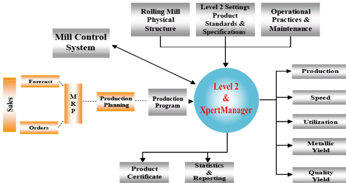
Figure 2. The Morgan XpertManager™ System Structure.
