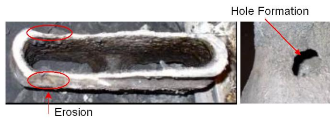
Fig. 7: Examples of Erosion on the Exterior of Nozzles From Off-Corner Vortexing
