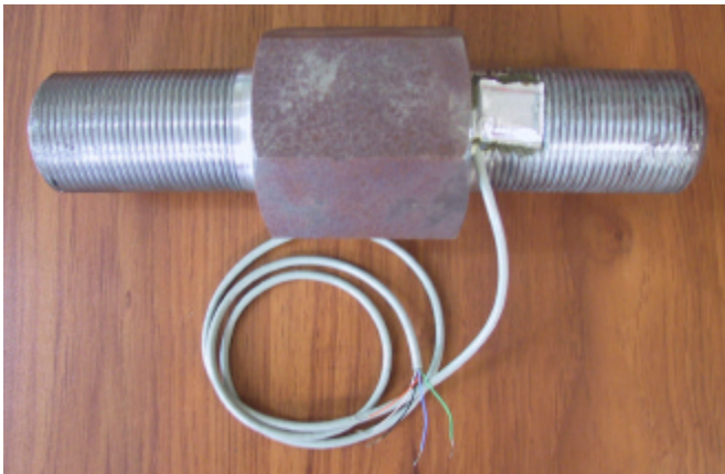
Figure 1. Cam rod after installing the strain gauge.
