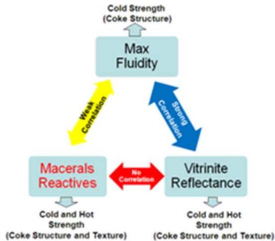
Figure 2. Relationships between coal quality characteristics and coke resistance – cold and hot.
