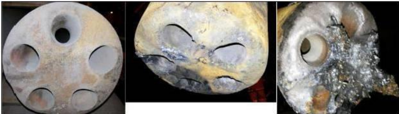
Fig. 8 - Nozzle wear and cartridge face due to differences between design conditions and operating conditions.
