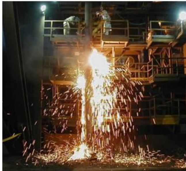
Fig. 4 - Vertical oxicut cleaning lance.
