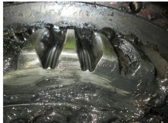
Figure 4. Gear spindle teeth wear.
