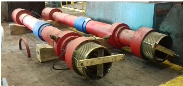
Figure 19. Spindles Ready for Installation
