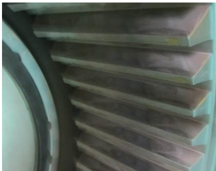
Figure 12. HSM Gear spindle components after 3 years of working.
