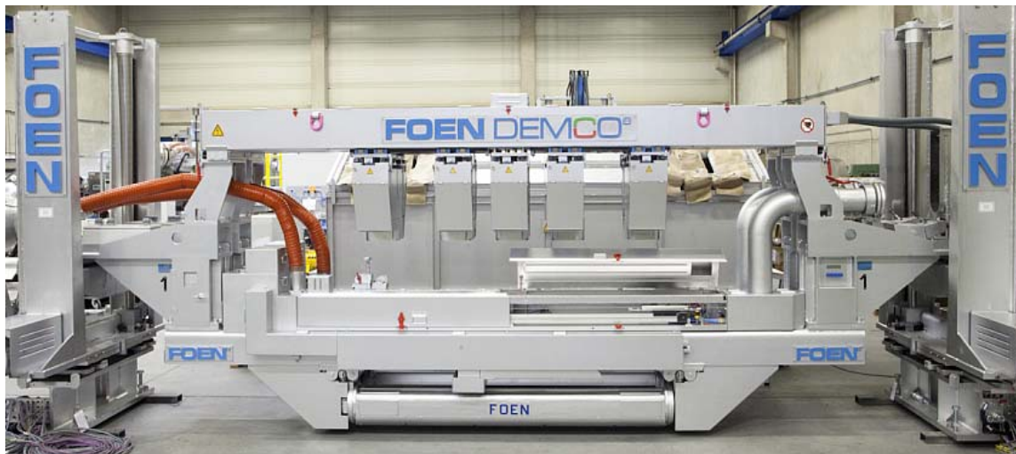
Figure 4. Moveable strip edge magnets to avoid lower overcoating.
