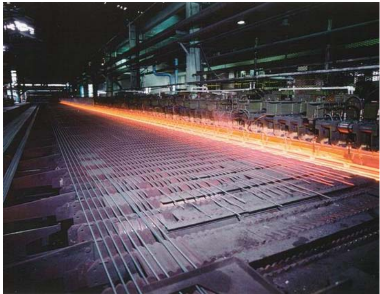
Figure 7 - Morgan High Speed Cooling Bed
