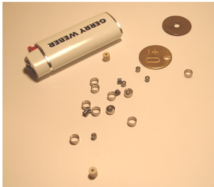
Figure 3. Sliding bearings for gyrocompass with monocrystalline carbon coating.
