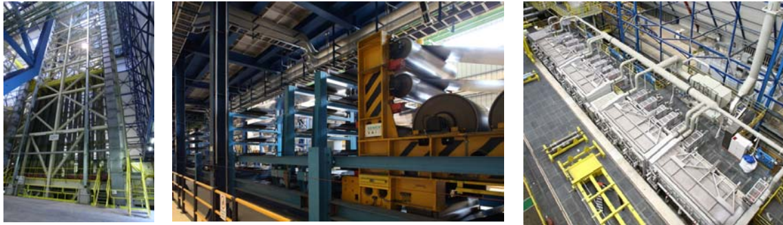
Figure 2. Vertical accumulator, horizontal accumulator, cleaning section.
