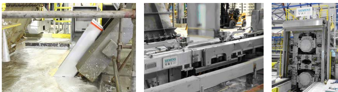
Figure 3. Zinc pot, wiping system and temper mill.
